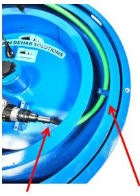
Insert the flex shaft cable into the ZIP ZIP holder then inside the connector and tighten by screwing.
