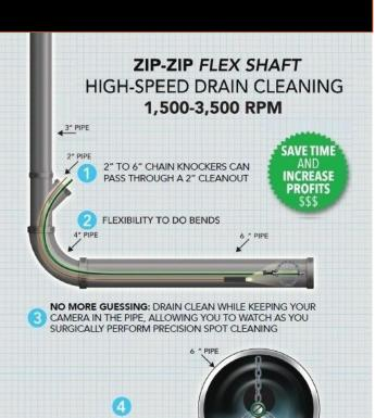
CHAIN KNOCKERS EXPAND TO FULL DIAMETER OF PIPE FOR 100% FULL CLEANING
