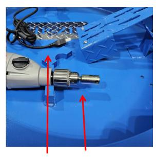
Insert the connector inside the drill chuck et tighten Ensure that the drill socket is not linked to the electrical power source.
