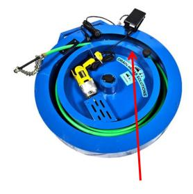
Plug the drill's socket into the switch foot pedal then plug the switch foot pedal socket into a power source
