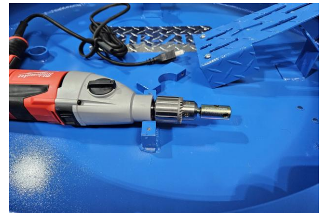
Insert the flex shaft connector inside the drill chuck and tighten the chuck
